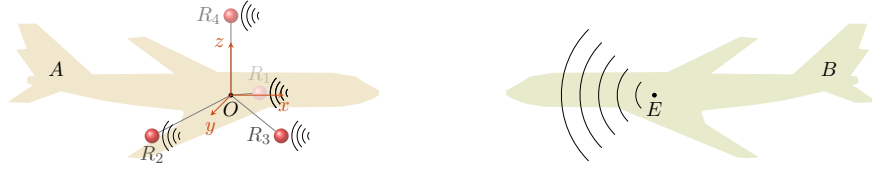
Figure 5: UAV A performing position estimation by listening for the single packet emitted by UAV B
